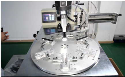
Ultrasonic Encapsulating For RFID Tag And Fobs
