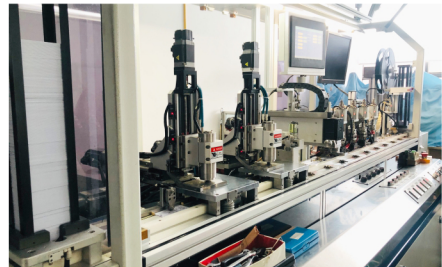
Smart Card Contact IC Chip Encapsulation
